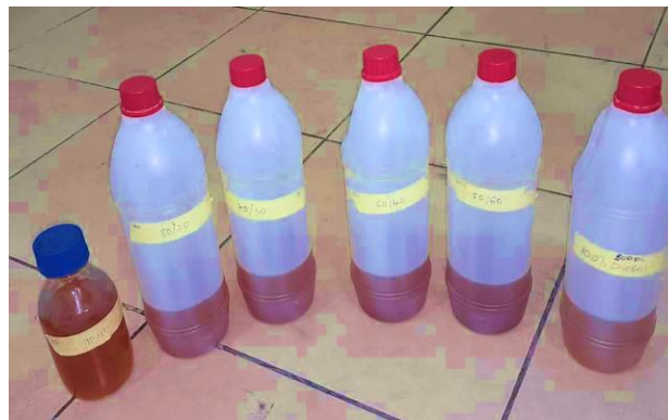
Figure 2: Blends of diesel and biodiesel. The biodiesel was synthesized from used cooking oil.
