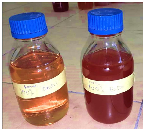
Figure 1: Samples of 100% diesel and biodiesel. Biodiesel was synthesized from used cooking oil.
